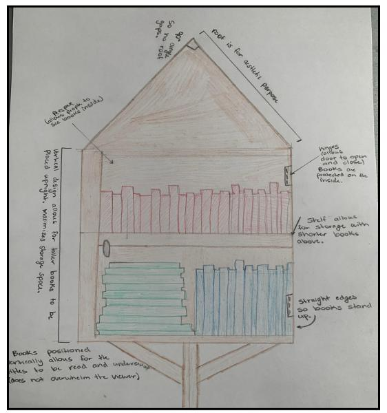
The chosen design has a square-like shape with a shelf on the inside. This design has a perspex door (so one may see the books inside), room for hardcovers to stand up horizontally, and is balanced on the support beams. This design uses the least materials for the highest amount of space while being aesthetically pleasing.
